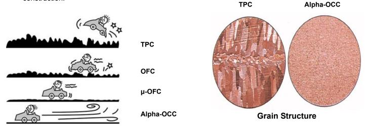
**TPC** (Tough Pitch Copper) is basic copper wire conductor typically found in power cords and occasionally inexpensive audio cables. Drawing melted, electrolyzed copper through a series of dies, the conductor is cooled to size. Tough pitch copper melted and cooled in "open air" carries about 300~500ppm of oxygen.
