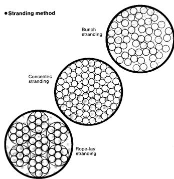
conductors form a perfect circle when viewed in cross section, improving performance by stabilizing impedance fluctuations.
